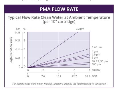
The micron ratings shown at various efficiency and beta ratio value levels were determined through laboratory testing, and can be used as a guide for selecting cartridges and estimating their performance. Under actual field conditions, results may vary somewhat from the values shown due to the variability of filtration parameters.
