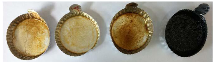
Figure 2: (Left to Right) Permeate samples from the V4, V5, V6 membranes, and feed.
