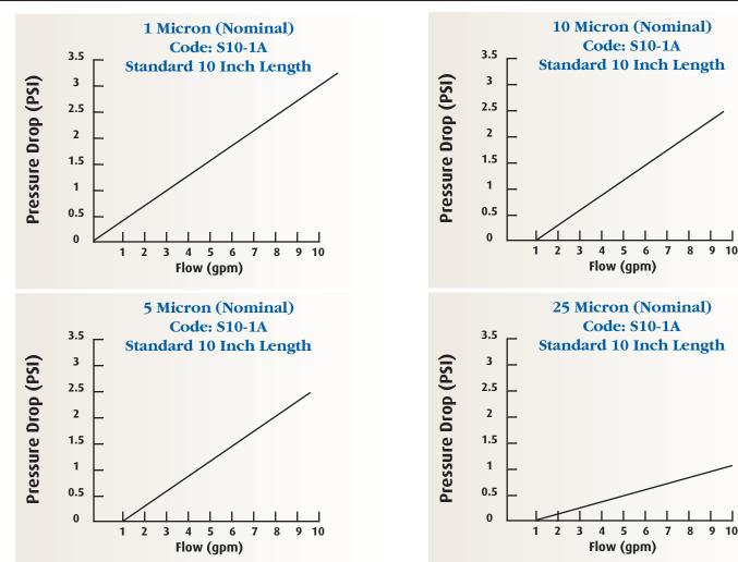
Test Fluid: Water at Ambient Temperature • Flow is in US Gallons per minute.
