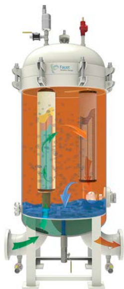
Figure 1. A typical two-stage vertical coalescer
